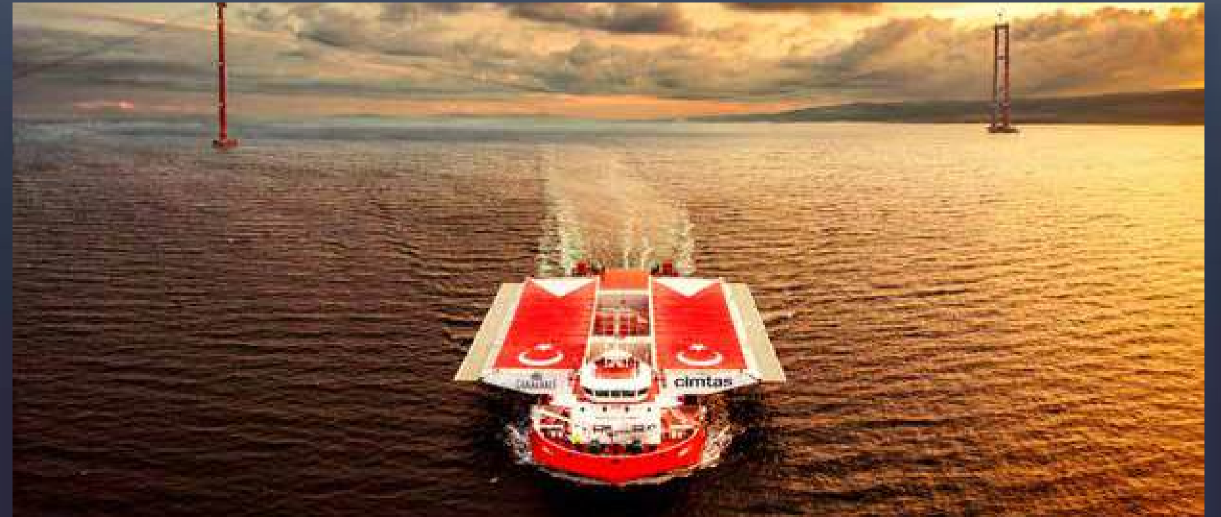
GIRDER BLOCK TRANSPORTATION
